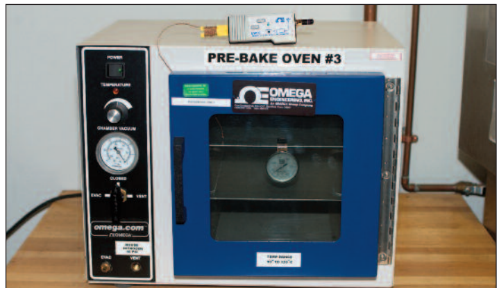
The wireless connector simplifies setup, and allows you to log data to a remote PC, up to 400' away.
